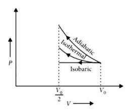
The P – V diagram of an ideal gas compressed from its initial volume  $V_0$  to  $\frac{V_0}{2}$  by several processes is shown in the figure.
