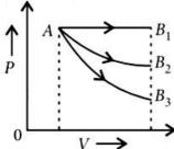
since area under  $\overrightarrow{AB}_1$ , is maximum, the work done is maximum in case of isobaric expansion.
